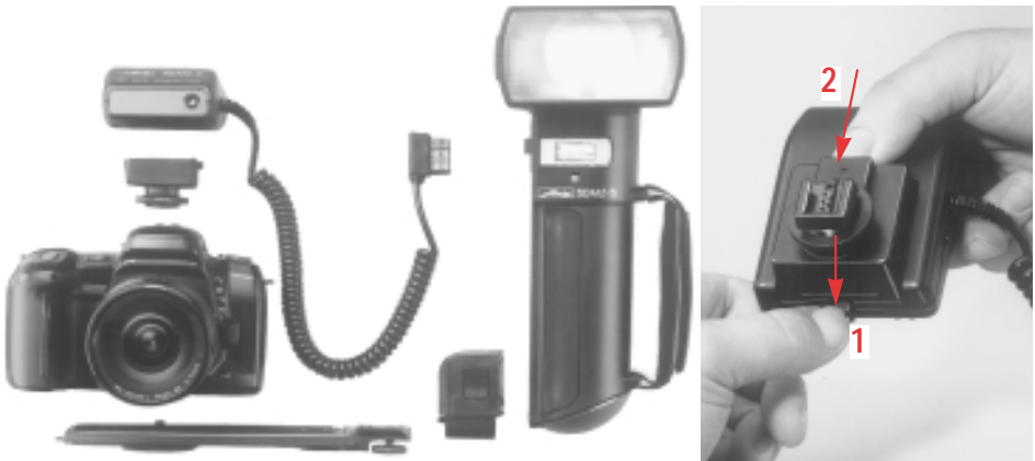
Fig. 1: Mounting the components, and removing the standard base or SCA adapter
